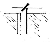
These windows can be made secure by drilling a downward sloping hole through the first sash, and one into (but not through) the second sash. Slide a nail or dowel into the hole.
